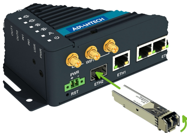
Figure 15: SFP Module Installation
