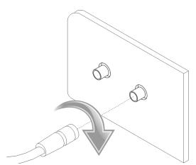
Figure 18: Connecting the antenna
