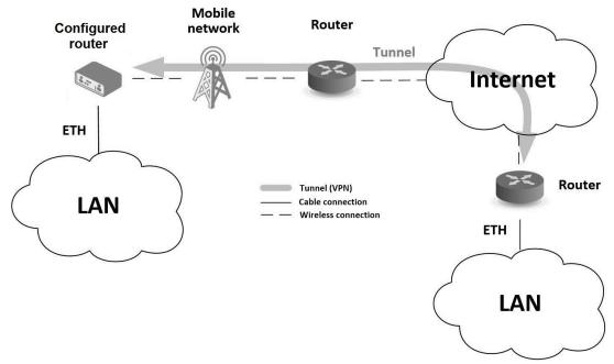
Figure 3: Using a VPN tunnel
