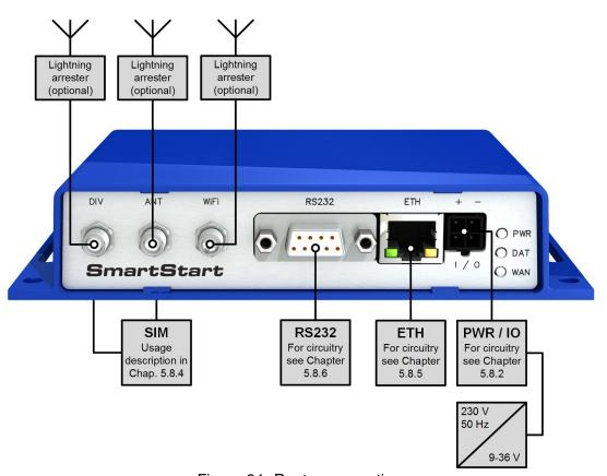
Figure 24: Router connection
