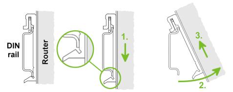
Figure 13: Removal from the DIN rail
