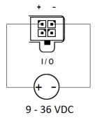
Figure 16: Circuit example - connection of power supply
